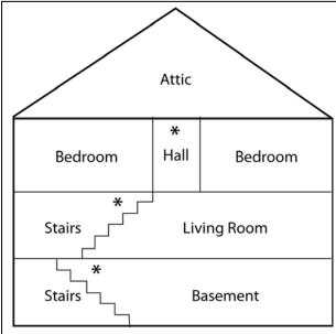
Install a smoke alarm and a carbon monoxide alarm (or combination alarms) in the basement and on each floor except the attic or a storage area.
